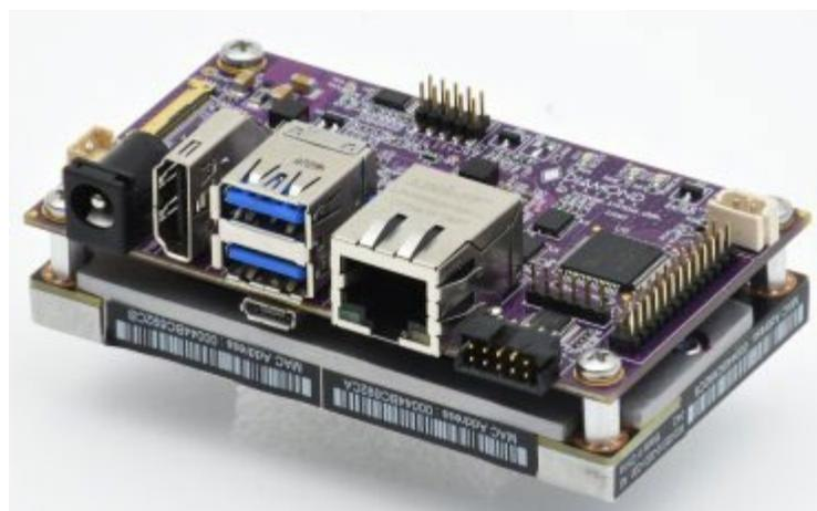
**Angle view with TX2 module installed underneath**
