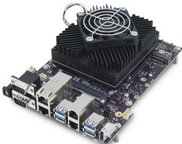
**Osbourne full kit with Orin module, fan sink, and commercial I/O adapter**
