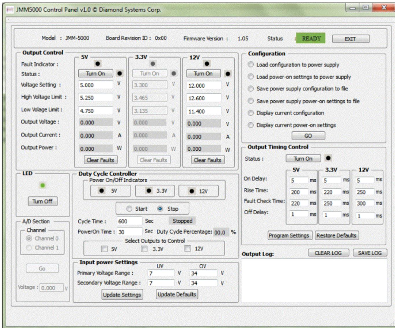
The intelligent models of JMM-5000 include a system controller that offers advanced configuration, control, and monitoring features. The system controller is accessed via a USB port and is accompanied by benchtop configuration software as well as an application library for in-application real-time control. Below is a list of key features included. More details can be found in the [Software user manual](#) and [Control panel user manual](#).
