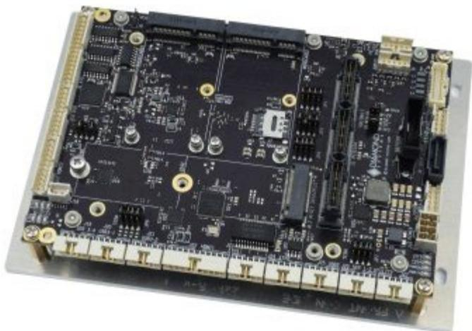
**Jasper SBC assembly with integrated mounting plate**
